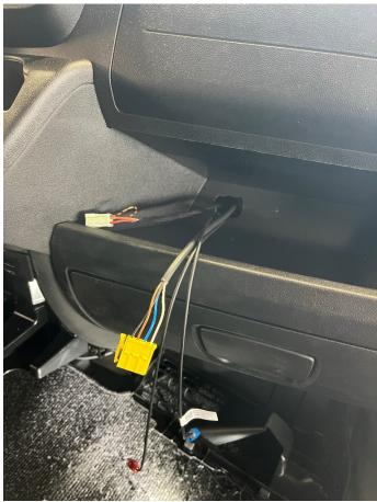
9. Pull the A plug cable from the passenger side to the driver's side. Lay the cable so that it is later behind the covers and can no longer be seen.
