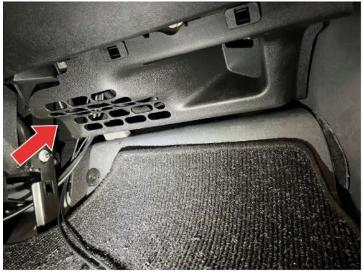
7. Then create a passage above the glove compartment and pull the KITAS sensor cable through.
