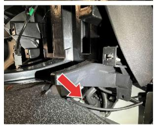
6. Remove the cover in the passenger compartment. This is only clipped on and does not need to be unscrewed.
