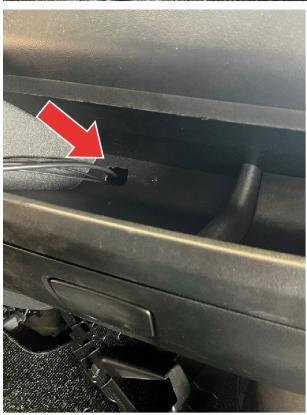
8. In addition, pull the DSRC cable and the cable with the A plug through the passageway.
