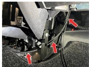
**10.** Remove the cover of the fuse box on the driver's side.
