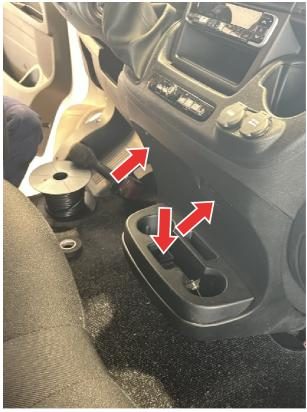
4. Unscrew the lower cover to be able to route the sensor cable into the vehicle interior later on.
